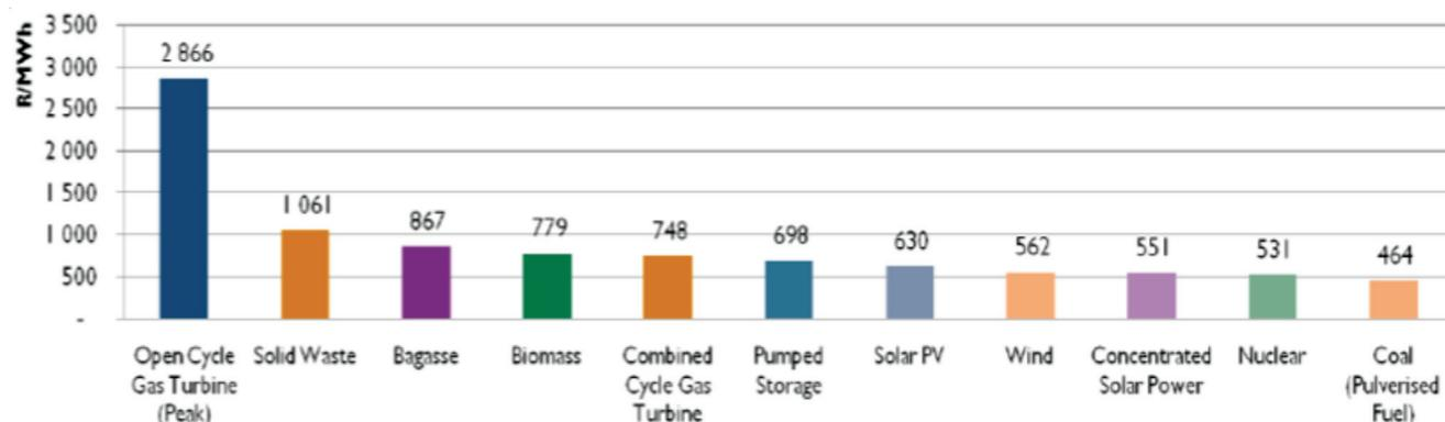
Figure 1. South Africa's IRP projected levellized cost of electricity in 2020 for various utility-scale generation sources (Department of Energy, 2011)
