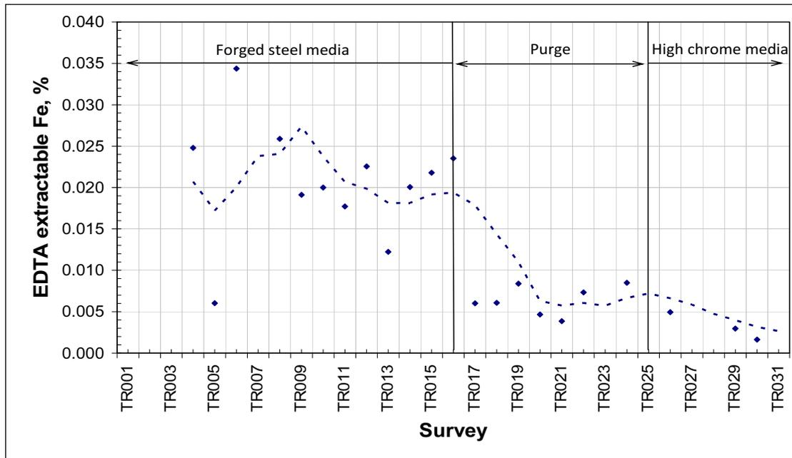
**Figure 2- The EDTA extractable iron trend with time for the primary rougher feed, moving from 100 per cent forged steel, through the purge period to 100 per cent high chrome grinding media. (TR refers to the pulp chemical survey number)**
