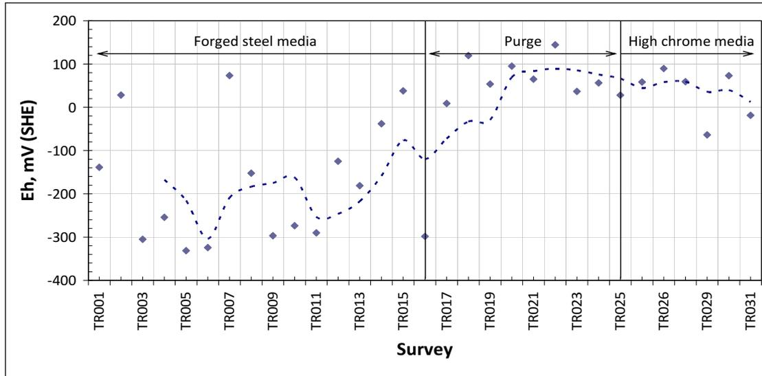
**Figure 1-The Eh trend with time for the primary ball mill discharge, moving from 100 per cent forged steel, through the purge period to 100 per cent high chrome grinding media. (TR refers to the pulp chemical survey number)**
