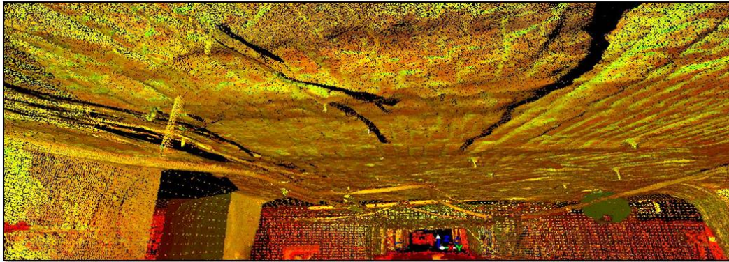
Figure 12-One scan reveals a vast amount of detail – support, geological features, Vent seals, etc.
