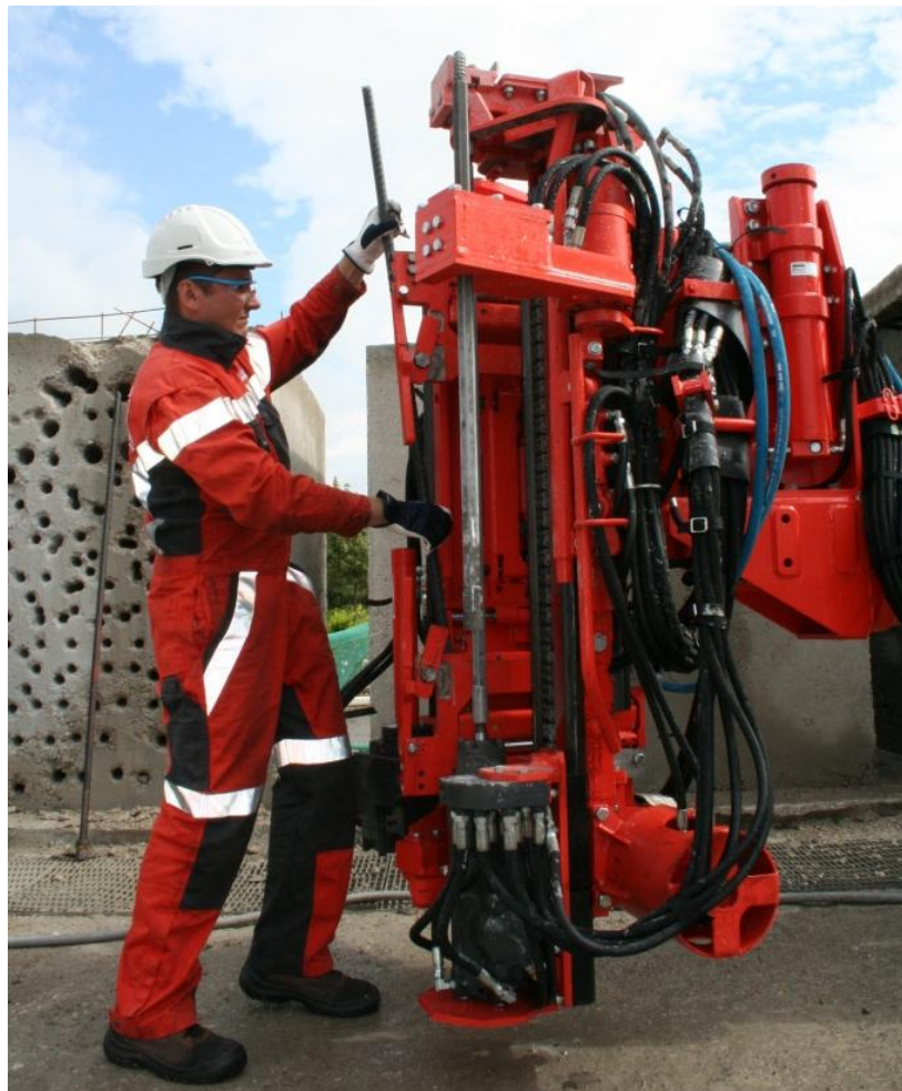
Figure 5-New TULPM bolting turret
