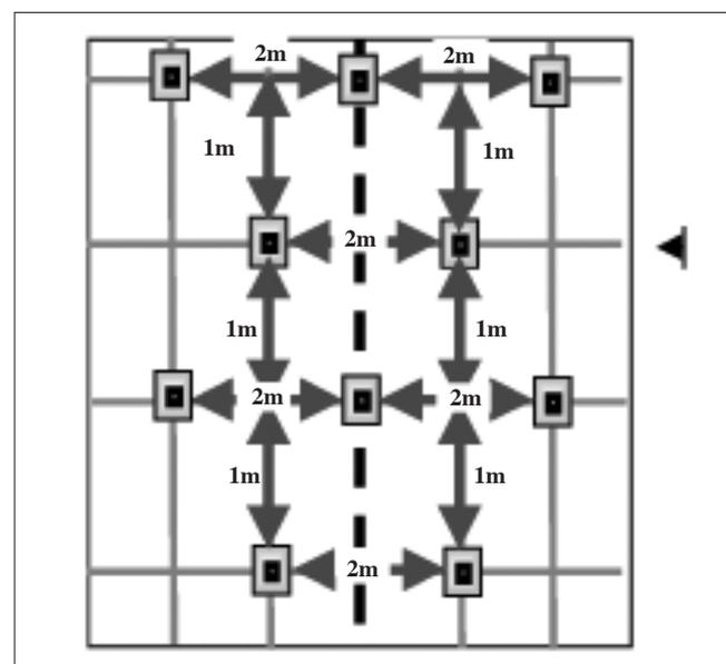
Figure 8. Stope support pattern at Two Rivers Platinum
