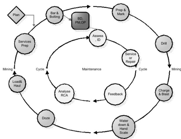
Figure 1. Continuous mechanized XLP cycle
