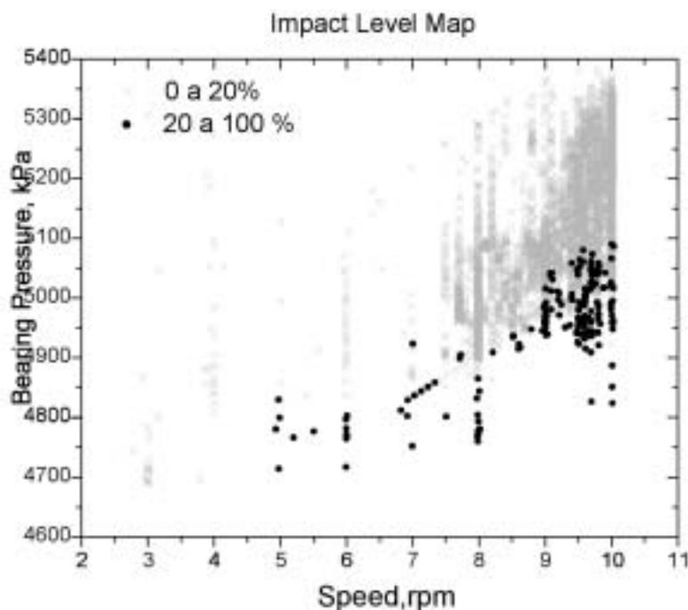
Figure 13. Impact level as a function of speed and bearing pressure
