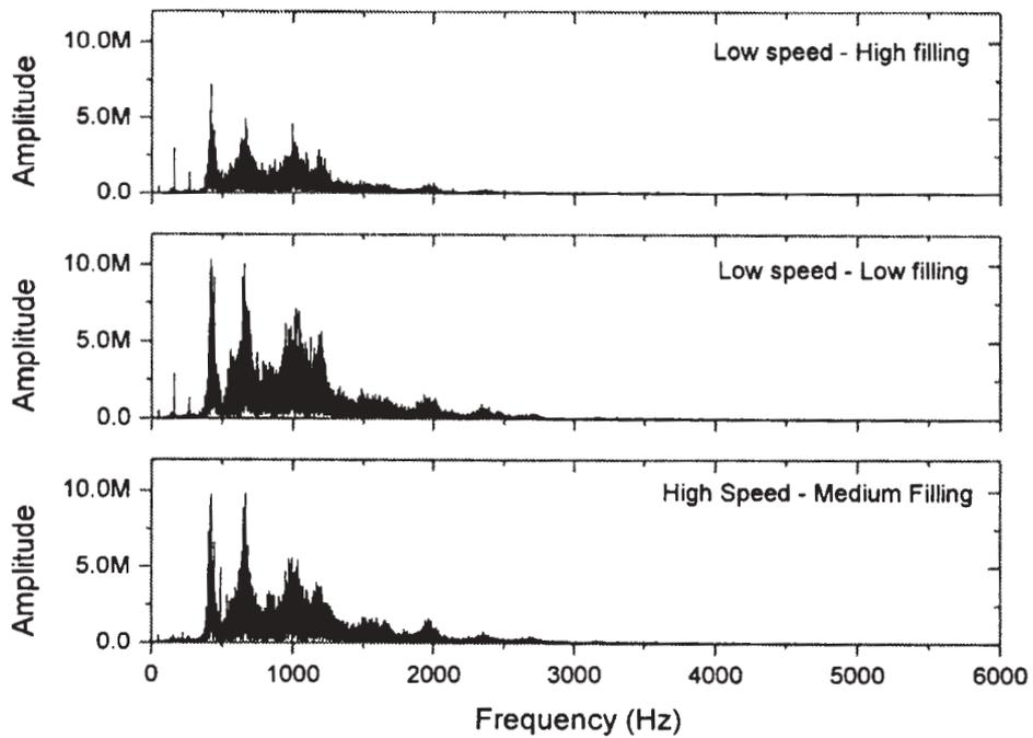
Figure 9. Samples of mill sound spectra, under low- and high- impact conditions
