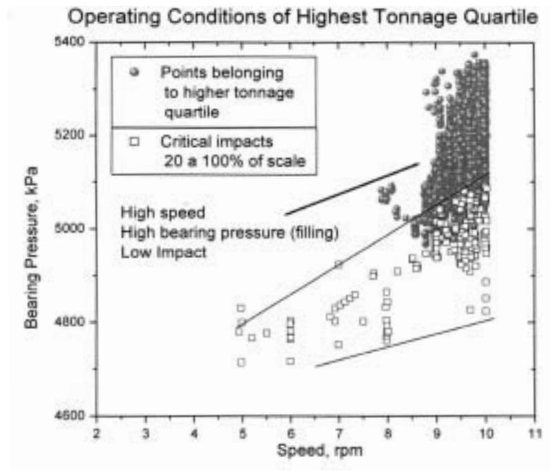
Figure 12. Inverse relationship between high tonnage and high critical impact
