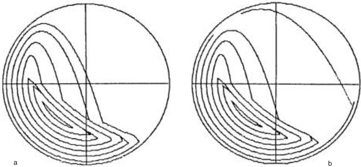
Figure 2. Schematic view of ball trajectories. Load falling onto itself (a) and on the liners (b)
