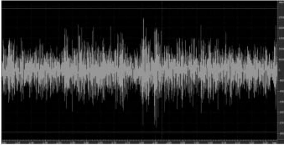
Figure 7. High-noise, associated with a low mineral hold-up condition as displayed by CoolEdit software and reflected as sound amplitude over time
