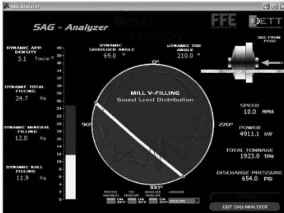
Figure 16. SAG analyser\*\* Monitor display
