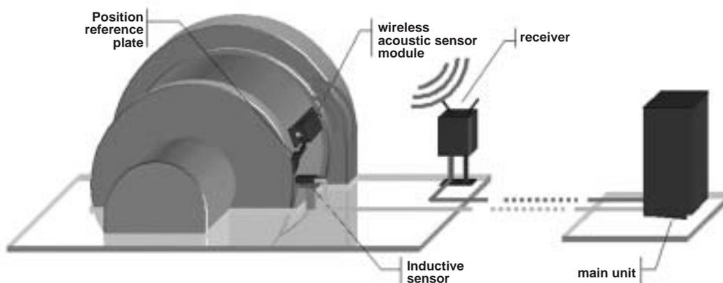
Figure 15. Layout of the microphone and position sensor in the mill
