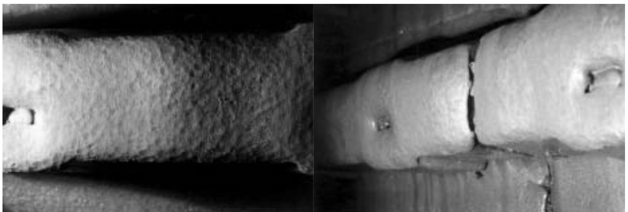
Figure 3. Examples of liner damage under impact
