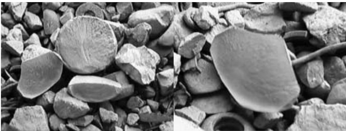
Figure 5. Excessive speed and low mineral hold-up cause extensive ball breakage
