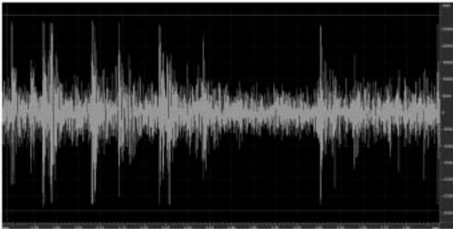
Figure 8. Impacts superimposed over mill noise as displayed by CoolEdit software and reflected as sound amplitude over time
