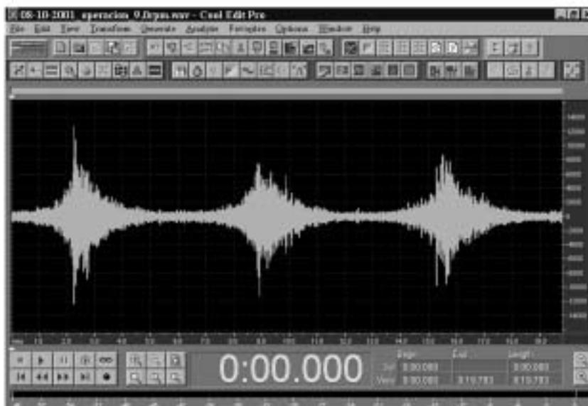
Figure 14. Sound trace used to find the charge position during a revolution of the mill. The toe is near the highest amplitude points
