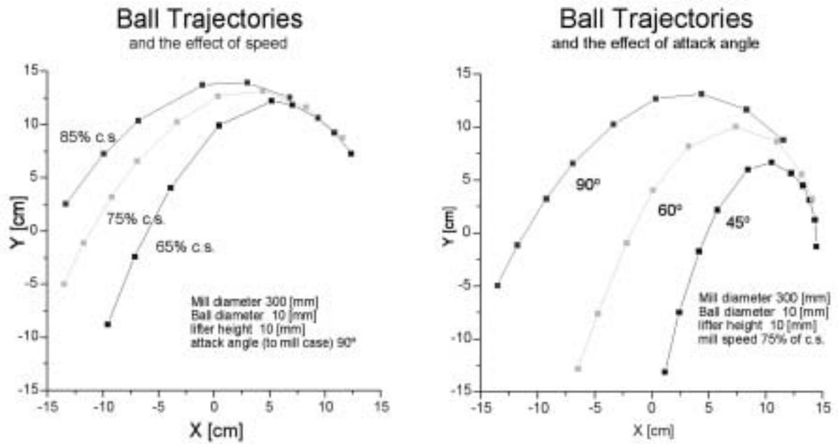
Figure 1. Effect of mill speed and lifter profile on load trajectories
