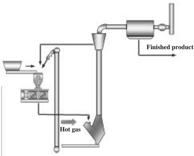
Figure 9. HPGR in dry grinding mode
