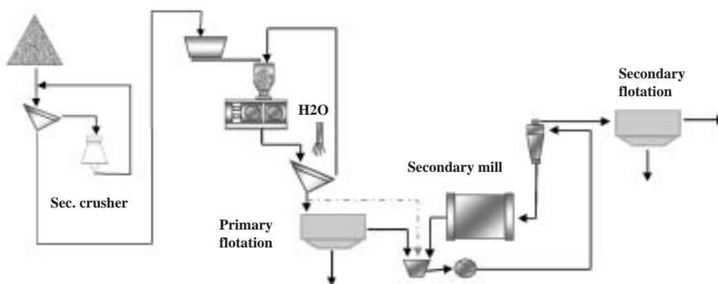
Figure 7. HPGR in closed circuit 'wet mode' (separating HPGR from the crushing circuit and combining it with the ball mill grinding plant)
