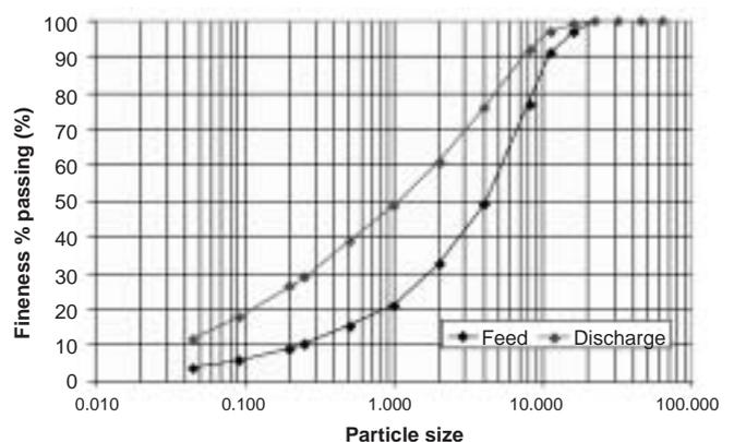
Figure 2. Expected size distribution for an industrial unit
