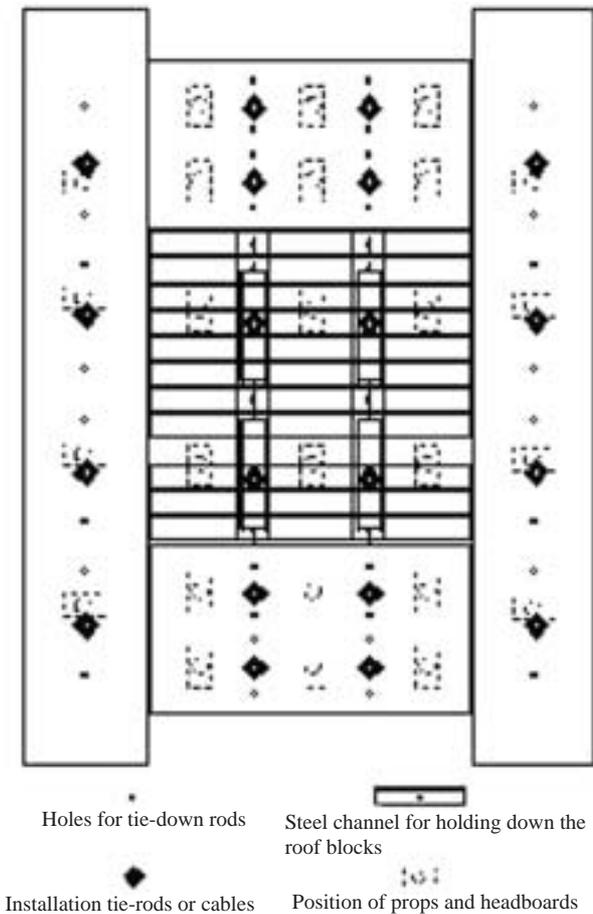
Figure 2. Plan view of the testing facility
