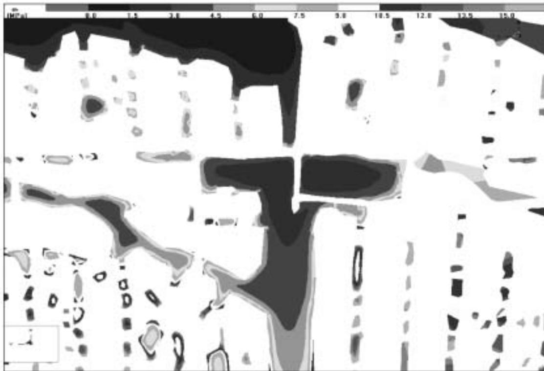
Figure 6. Results—contour plot of pillar stress (MPa)
