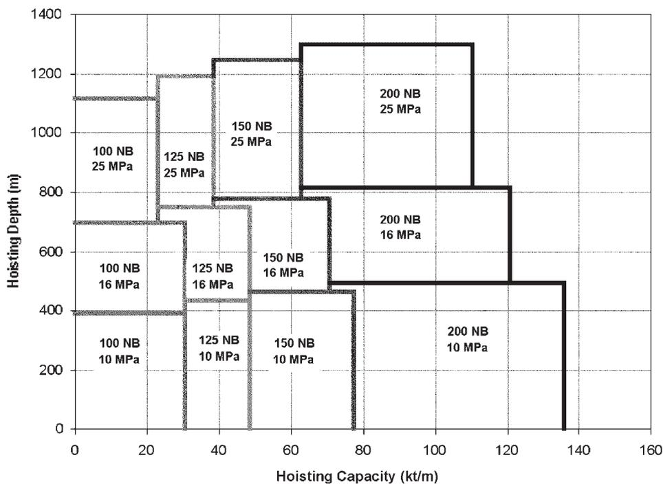
Figure 9. Hydraulic hoisting system selection chart (UG2 Ore)
