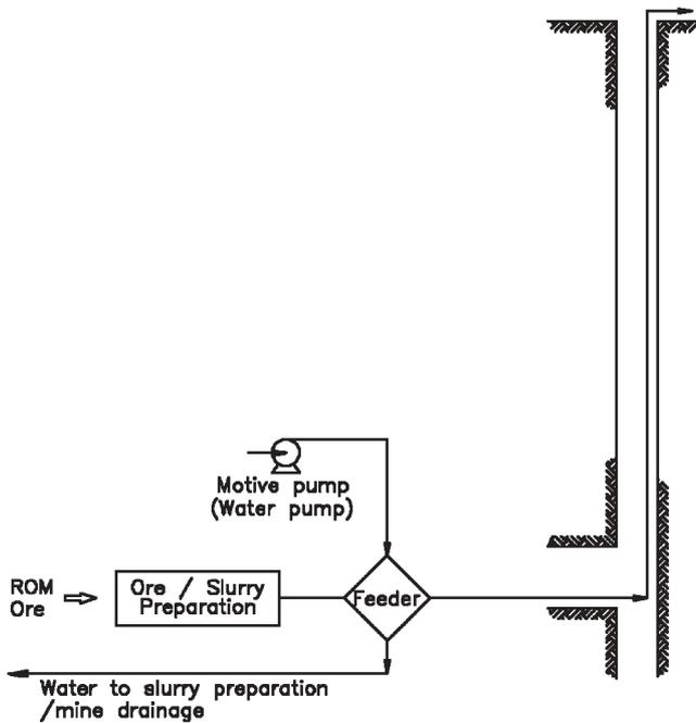
Figure 5. Feeder system with motive water pump underground
