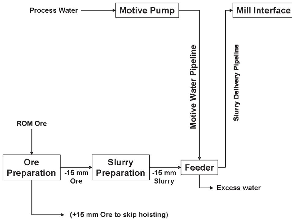
Figure 8. Typical hydraulic hoisting system flow sheet
