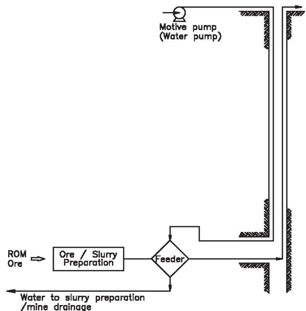
Figure 4. U-tube type feeder system
