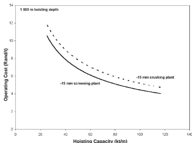
Figure 11. Hydraulic hoisting system operating costs
