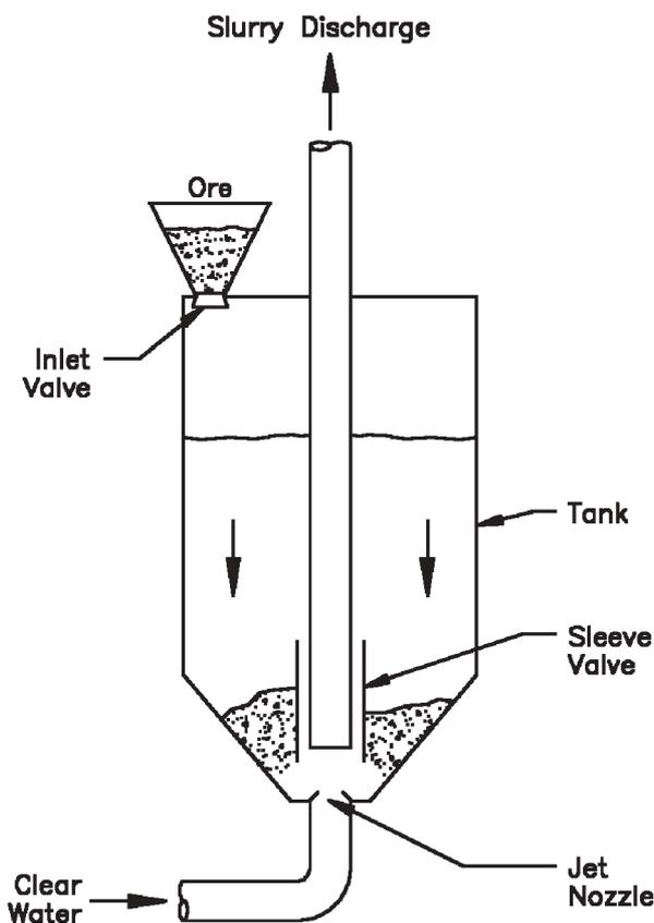
Figure 6. Hydro-lift feeder
