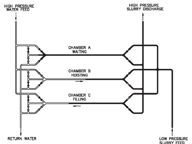
Figure 7. Three-chamber pipe displacement feeder
