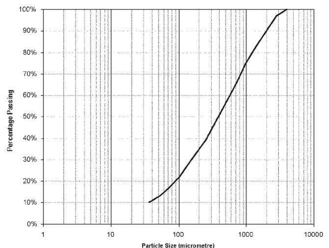
Figure 2. Upper particle size grading limit for piston diaphragm pumps
