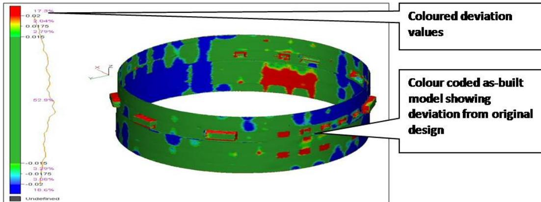
Figure 6-Shaft alignment
