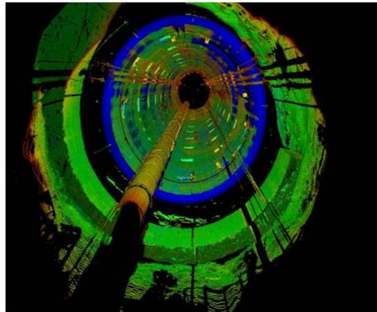
Figure 8-Scan (green) compared with design (blue)
