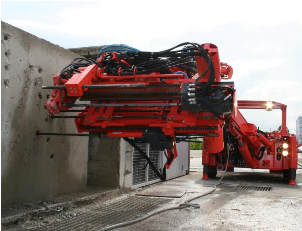
Figure 4-Mechanized roofbolter (DS210L-M) with new TULPM turret
