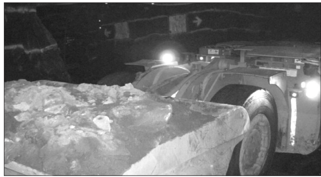
Figure 7. LP LHD (ASD loading and ore removal)
