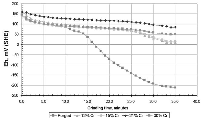
**Figure 5.** The Eh profile during grinding for each grinding media type for tests completed on a UG2 ore
