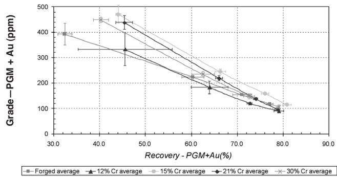
**Figure 6.** PGM+Au grade/recovery curves for laboratory rougher flotation tests completed on UG2 ore ground with forged, 12, 15, 21, and 30 per cent chrome grinding media
