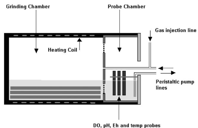
Figure 3. Schematic representation of the Magotteaux Mill®
