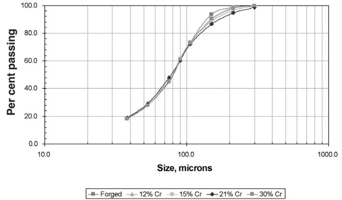
**Figure 4.** Particle size distribution data a UG2 ore ground with forged steel, 12, 15, 21 and 30 per cent chrome grinding media
