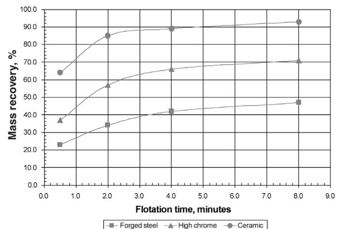
**Figure 2.** Mass recovery versus flotation time curves for rougher flotation tests completed on 100 grams of Rapid Bay galena ground to a  $P_{50}$  of 9 microns using forged steel, high chrome, and ceramic media. The tests were completed in demineralized water (pH 7), and employed 1 000 grams per tonne of sodium ethyl xanthate collector
