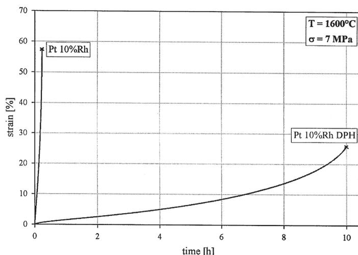
Figure 7. Creep curves of Pt 10%Rh and Pt 10%Rh DPH at 1600°C,  $\sigma = 7$  MPa
