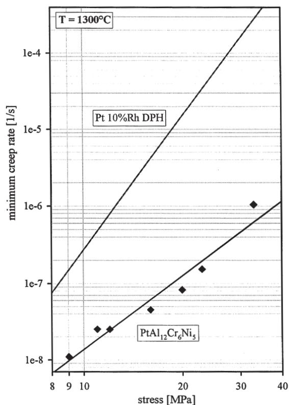
Figure 11. Norton plot of Pt 10%Rh DPH and PtAl<sub>12</sub>Cr<sub>6</sub>Ni<sub>5</sub> at 1300°C
