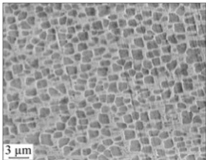
Figure 3. SEM micrograph showing two-phase  $\gamma/\gamma'$ -microstructure of Pt-base superalloy PtAl<sub>12</sub>Cr<sub>6</sub>Ni<sub>5</sub>
