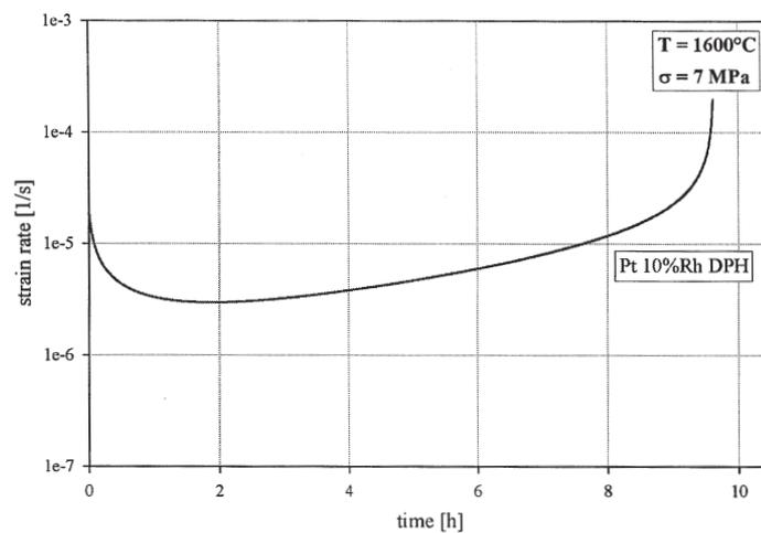
Figure 9. Creep rate of Pt 10%Rh DPH at 1600°C, calculated from the creep curve in Figure 7
