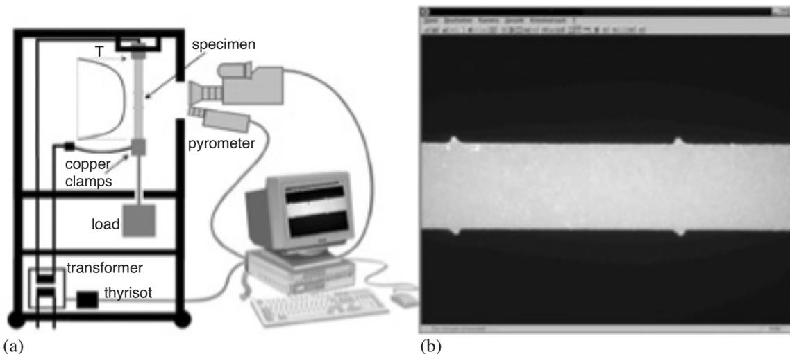
Figure 4. (a) Creep testing facility for tests at constant load either in air or inert gas atmosphere at temperatures up to 3000°C. (b) Screenshot of the software SuperCreep for strain measurements.
