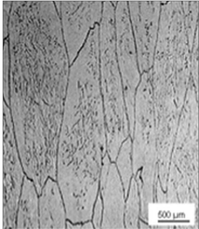
Figure 2. Optical micrograph showing the microstructure of internally oxidized Pt DPH
