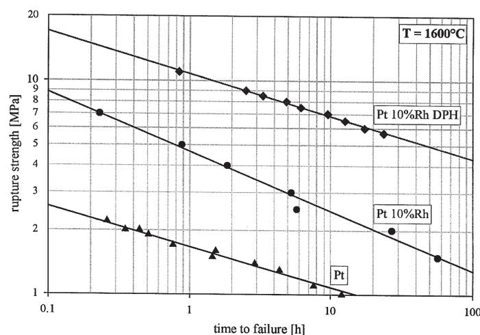
Figure 5. Stress-rupture strength curve of Pt and Pt-alloys at 1600°C
