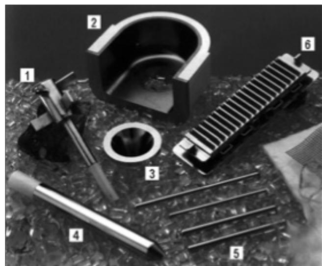
Figure 1. Components made from platinum for the glass industry: (1) stirrer, (2) spout bowl, (3) drain bushing, (4) plunger, (5) thermocouple thimbles, (6) bushing
