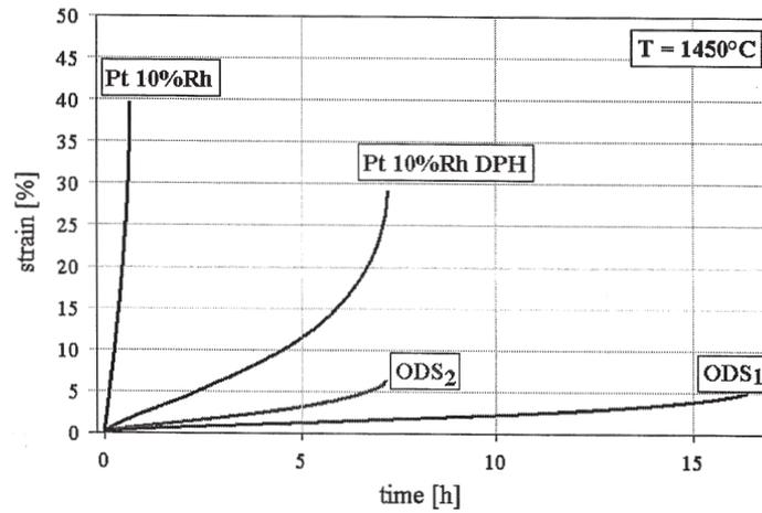
Figure 8. Creep curves of several platinum alloys at 1450°C
