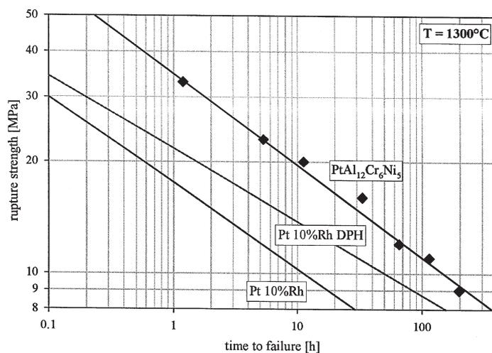
Figure 6. Stress-rupture strength curve of different Pt materials at 1300°C
