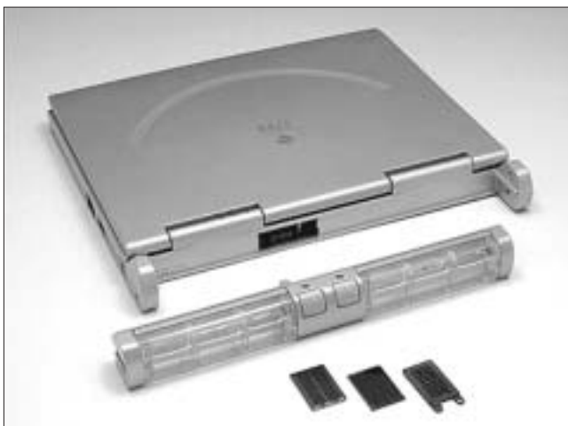
Figure 11. A laptop powered by a DMFC
