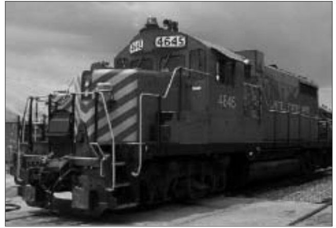
Figure 8. A 109-ton diesel-electric locomotive fitted with a 1.2 MW fuel cell
