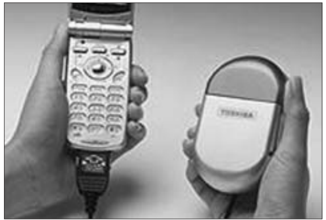
Figure 10. A GPS powered by a DMFC
