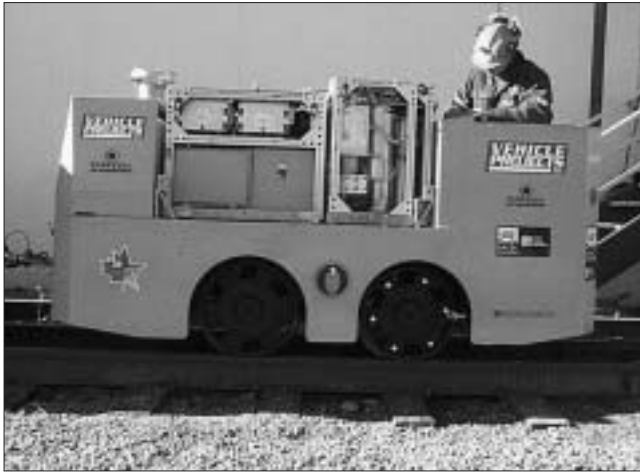
Figure 7. An underground mining fuel cell locomotive
