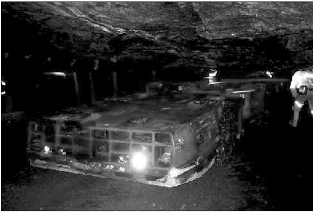
Figure 2. Severe damage to machine extremities from undulating floors and mechanical contact with roof in an extra low profile stope (EJC 88XLP)
