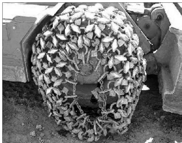
Figure 8. Typical chain failure. The chain has slipped off the tyre
