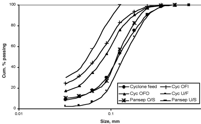
Figure 11. Particle size distributions for the three-product cyclone and Pansep screens obtained from the pilot plant tests
