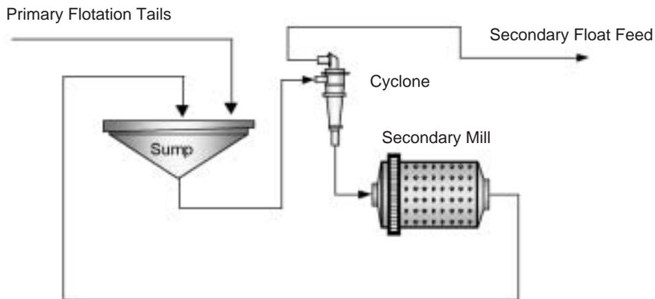
Figure 4. Secondary mill schematic: closed circuit operation
