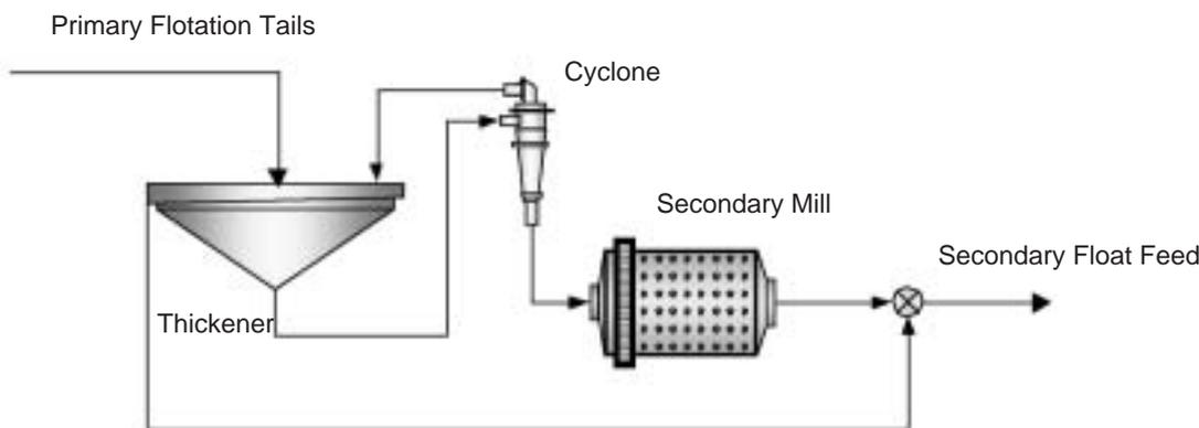
Figure 5. Secondary mill schematic: open circuit operation
